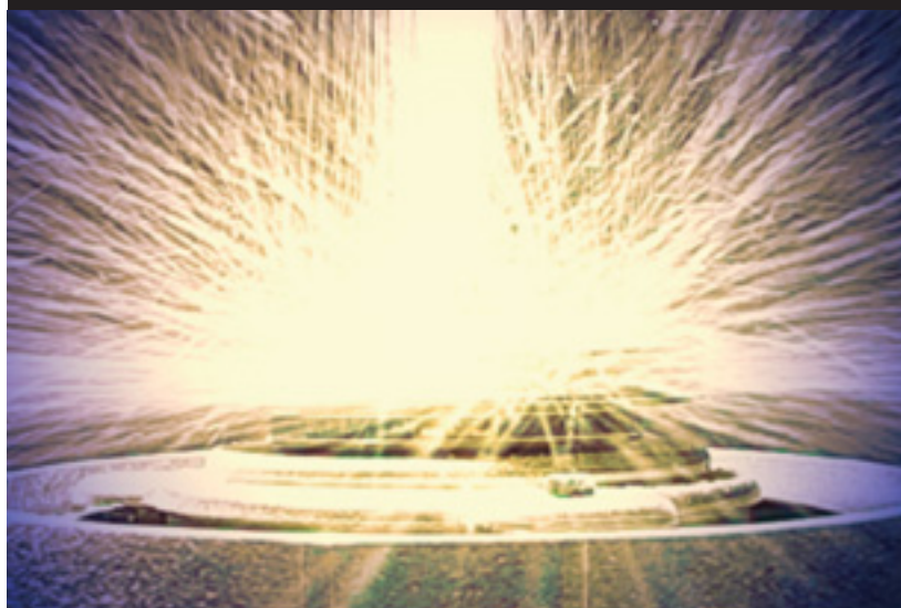
High speed photos depicting the bladed rotor at the moment of impact with cascading dry polymer stream. The increasing particle angular velocity imparted by the rotor, is rapidly intensified to over 3600 feet per minute – prompting frequent collisions and uniform polymer separation prior to wetting.
